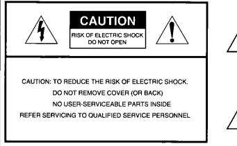
The lightning flash with arrowhead within a triangle is intended to tell the user that parts inside the product are a risk of electric shock to persons.
